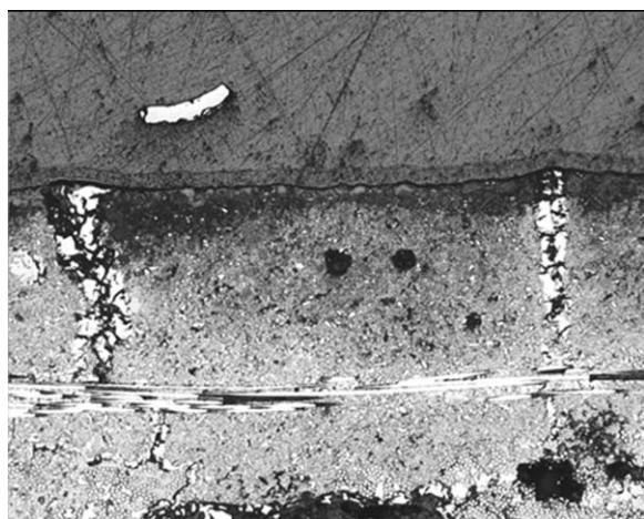
Fig. 10. Bonding crack formation during pyrolysis and further filling by PIP.
